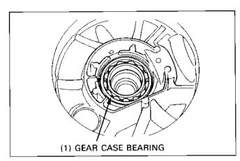
Install the oil seal remover into the gear case bearing.
