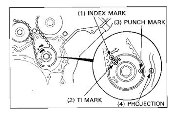
Align the T1 Mark on the drive pulley guide plate with the Index Mark on the crankcase.
