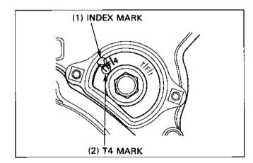
Make sure that the <u>Punch Mark</u> on the driven pulley aligns with the <u>Index Mark</u> on the reduction holder. If not, turn the crankshaft clockwise one full turn and realign the <u>T4 Mark</u> with the Index Mark.
