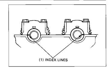
Install the dowel pins and camshaft holders.
