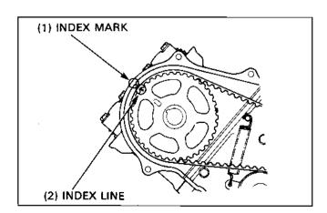
Install the intake and exhaust camshafts so that the <u>Index</u> <u>Lines</u> on the end of the shafts are facing outward and that they align with the top of the cylinder head as shown.
