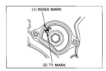
Make sure that the Index Line on the driven pulley aligns with the Index Mark on the reduction holder. If not, turn the crankshaft clockwise one full turn and realign the T1 Mark with the Index Mark.
