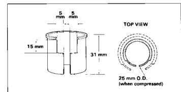
Tappet hole protector; an equivalent tool can be made from a plastic 35 mm film container using the measurements shown above.
