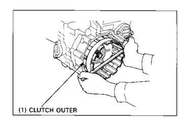
Turn the oil pump driven sprocket with a screwdriver as shown while pushing the clutch outer in until you feel a click. At this time, the holes in the clutch outer are aligned with the pins on the oil pump drive sprocket. Push in the clutch outer further to insert the pins into the holes.
